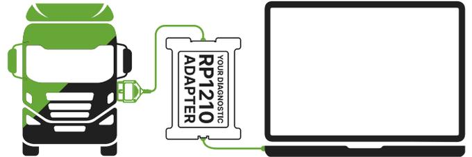
2. Connect **ONLY** the **RP1210** adapter to your laptop and the **OBD** socket in the cab.
