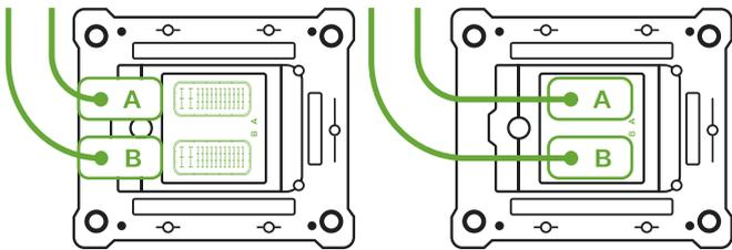
1. Connect both harnesses (**A,B**) to the **ECM/EMS** module on your truck.
