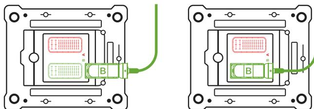
2. Connect the **VLOMINGO** adapter to the "**B**" socket on the **ECM/EMS**.
